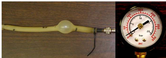
Figure 45: Bubble formation accompanied by drop in pressure
