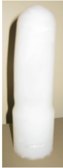
Figure 17: \alpha -prototype created using a curable silicon cast in an expendable wax mold
