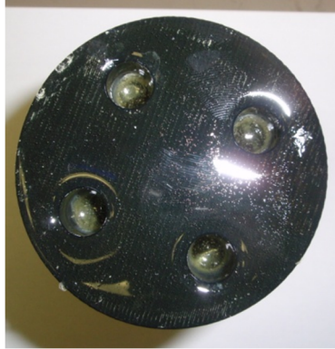
Figure 14: Assembled mold with PU \alpha inside, photograph was taken after vacuum pump was used and the curing process was finished
