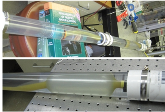
Figure 42: Series accumulator configuration (top); Bladder inflation within a fluid-filled shroud (bottom)
