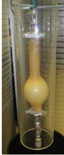
Figure 23: 1" ID 3/2" OD LX \alpha tube expanding without coming into contact with the 6" ID PC shroud
