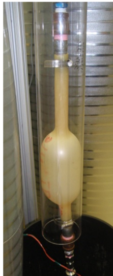
Figure 24: 1" ID 3/2" OD LX \alpha tube expanding such that the 3.75" ID PC shroud limits its radial expansion
