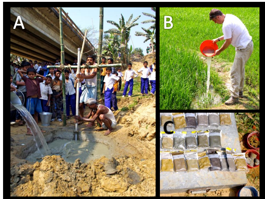
Figure 6: (A) Fulcrum-and-lever drilling method. (B) Drill fluid being decanted off sediment. (C) Bagged samples after color and grain size description.
