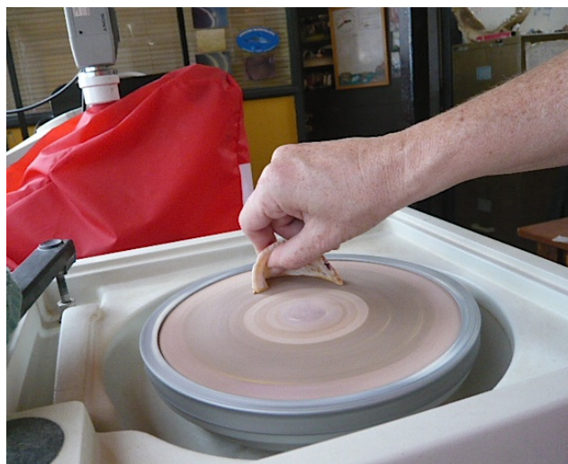
Figure 4.5: Section of a cut shell of C. concholepas being polished using a machine prepared with Brasso, a liquid polishing product used to highlight the growth lines.
