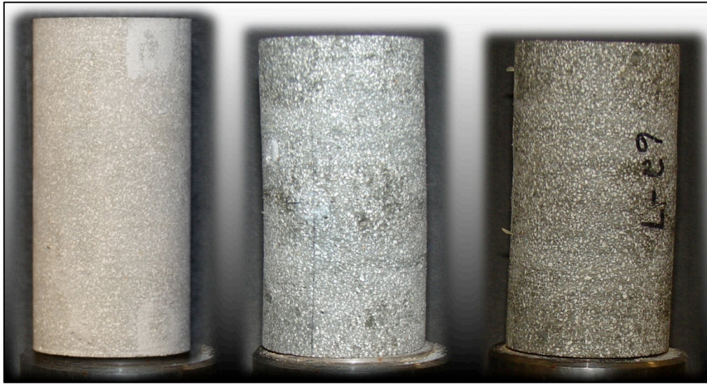
Figure 4.15 UXC specimens: before test (left); after test 5 (middle); after test 6 (right)
