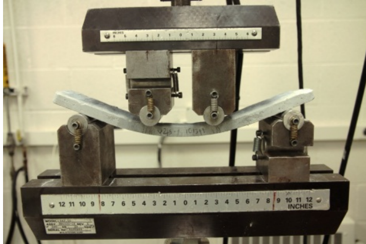
Figure 2.5 HSHDC loaded in flexure
