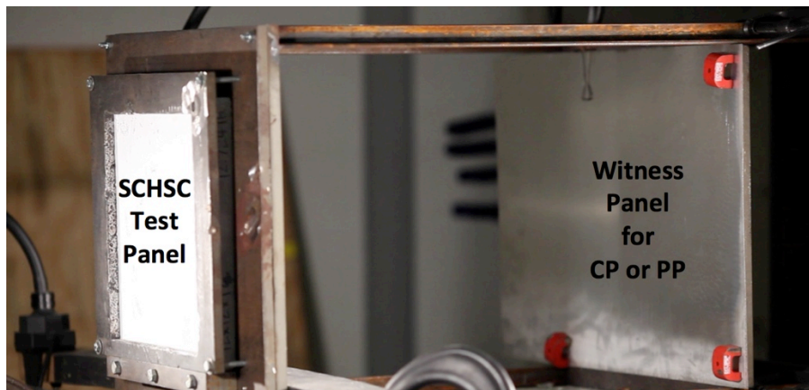
Figure 6.4 SCHSC panel mounted with witness panel for ballistic evaluation
