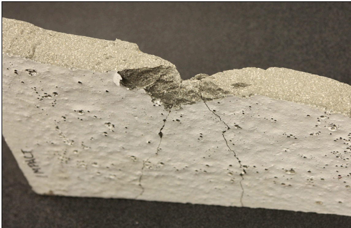
Figure 6.9 Typical cross section showing overlap of impact and exit craters for all panels in Test series #1 (25mm: No fibers)
