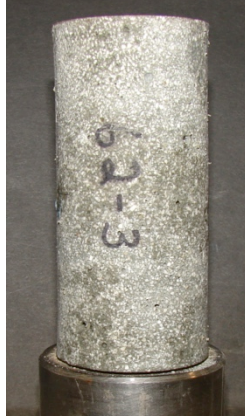
Figure 4.12 Specimen after the HC experiment was completed (no visible damage)
