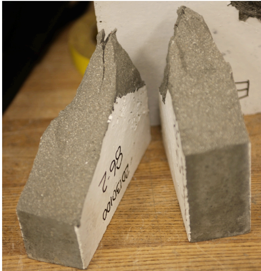
Figure 6.15 Portions of two different target panels from Test series three showing intersection of impact and exit craters indicating no projectile tunneling occurred
