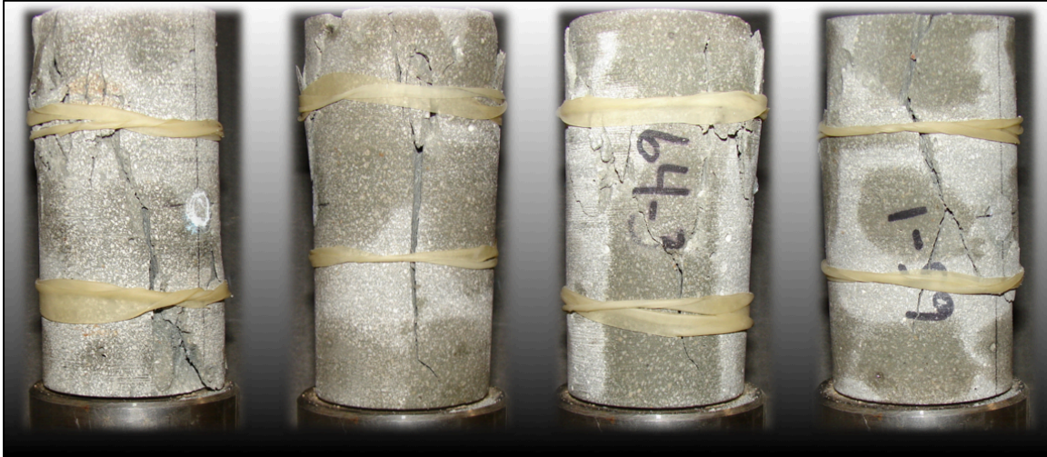
Figure 4.19 Specimens at failure for UC test 1 (left); UC test 2 (left-middle); UC test 3 (right-middle); and UC test 4 (right)
