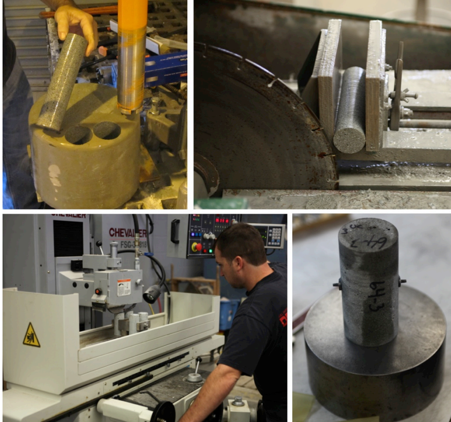
Figure 4.1 Coring (top left), sectioning (top right), precision grinding (bottom left), and a final specimen used for the hydrostatic, triaxial or uniaxial strain experiment
