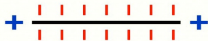
Figure 3.5 PPNC particles are negatively charged along axis and positively charged on the ends
