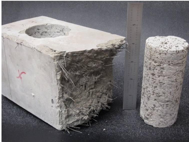
Figure 3.30 Specimen cored from beam to evaluate fiber distribution using MicroCT
