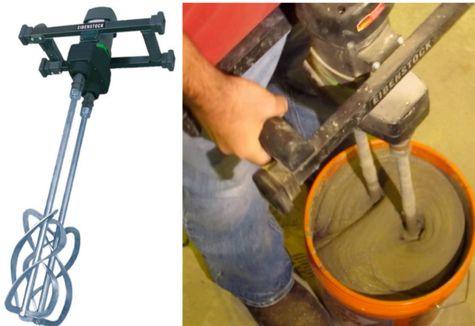
Figure 3.7 Mixing with Eibenstock 21 S twin paddle concrete mixer
