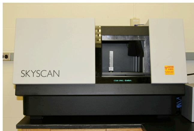
Figure 3.9 Concrete specimen mounted in the SkyScan 1173 X-ray micro-CT device
