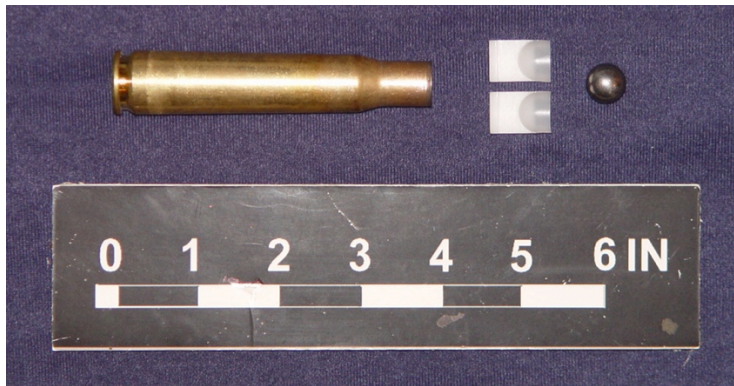
Figure 6.5 Cartridge with plastic sabot and 12.7mm spherical projectile
