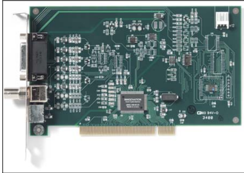
Figure 4: CyberOptics Imagenation PXC-200 series PCI frame grabber [20]
