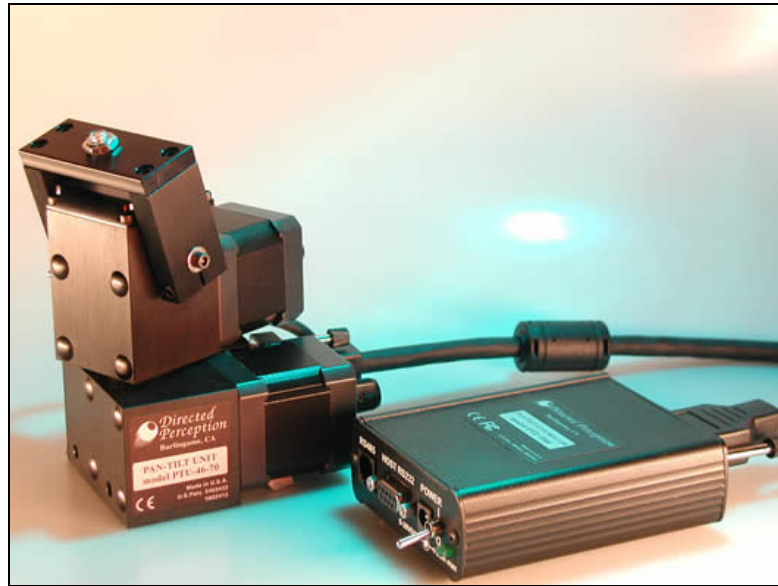
Figure 3: Directed Perception PTU-46 series pan-tilt unit with controller [18]
