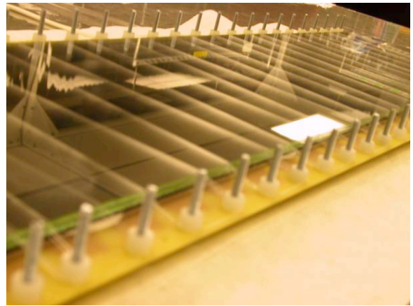
(A) Open MRPC chamber with stack of glass plates separated by fishing line
