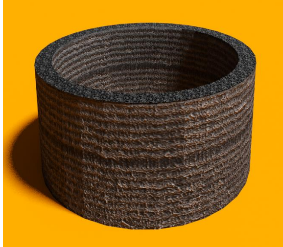
Figure 7.3 3-D model of a PSi microcavity ring resonator.
