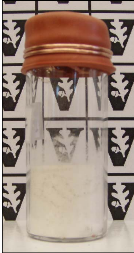
Figure 2.12 A 10-mL de-aggregation vessel charged with approximately 5 mL of ZrO 2 grinding media and sealed with a rubber septum and copper wire.
