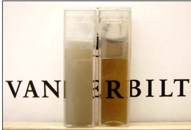
Figure 2.10 Solutions of UDD (left) and ND (right) in DMSO. The concentration of each sample is approximately 0.25 weight %.
