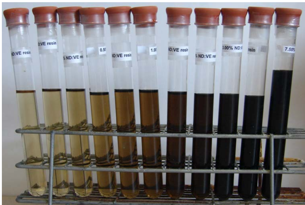
Figure 5.6 Uncured VE resins containing ND-VTMS filler up to 7.5 weight percent. The concentration of nanodiamond, from left to right, is 0.00, 0.10, 0.25, 0.50, 0.75, 1.00, 1.50, 2.00, 3.00, 5.00, and 7.00 wt percent.
