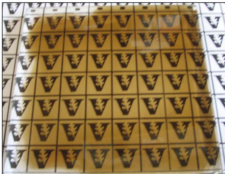
Figure 5.16 An uncured vinyl ester film containing 1.2 volume percent ND-VTMS showing excellent optical transparency.
