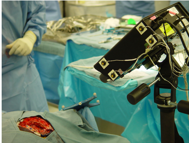
Fig.IV.1: shows a laser range scanner acquiring data in the operating room. The height and angle of the scanner are both adjustable. A built-in digital camera inside the scanner acquires high resolution digital images immediately after the range data has been acquired.
