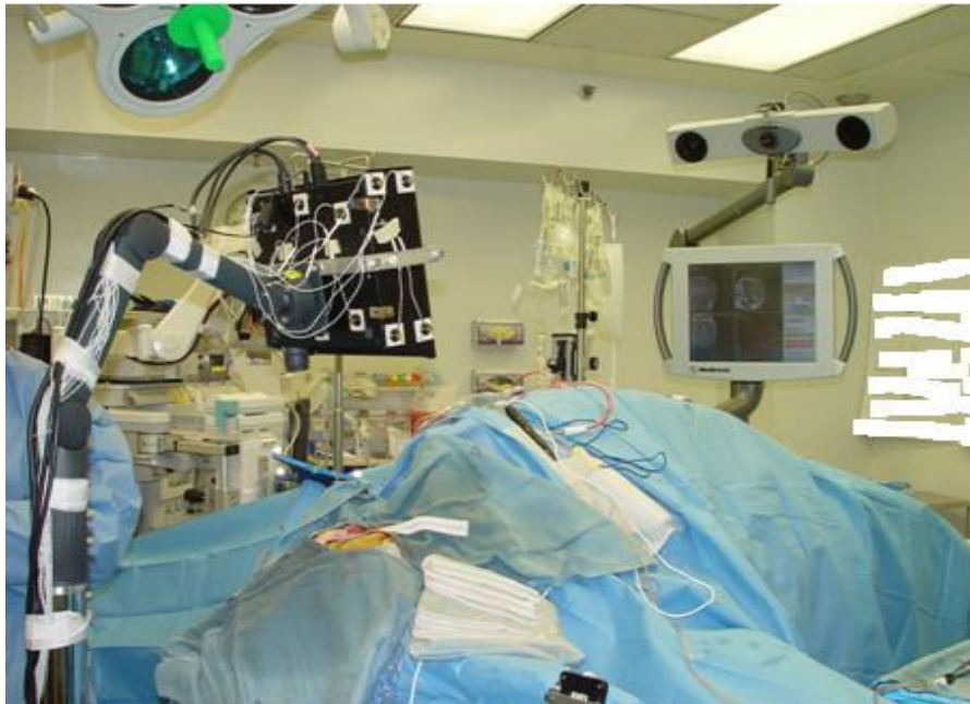
Fig.II.1: View of the operating room with the tracked laser range scanner positioned approximately 30cm above the craniotomy.
