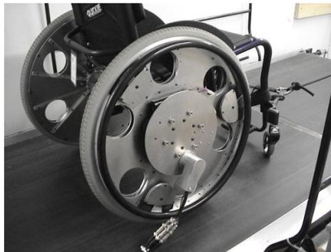
Figure 1.4 The wired version of MAX Mobility's propulsimeter.
