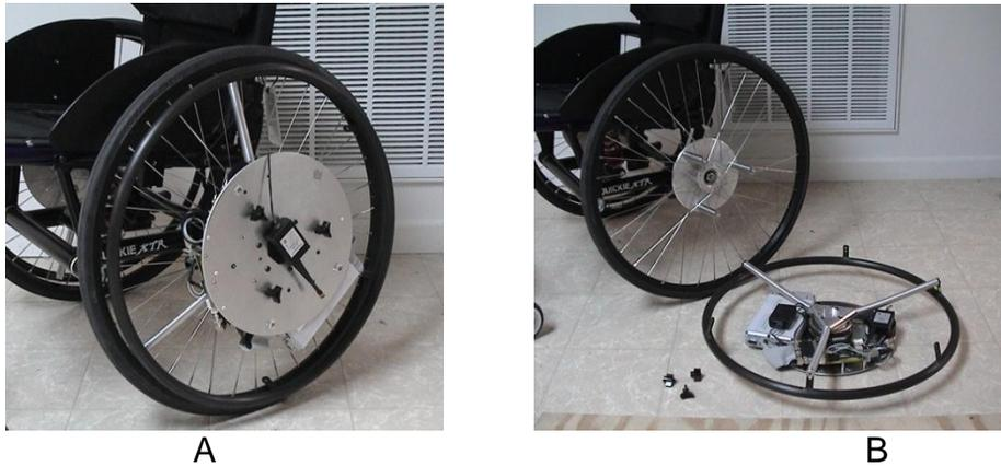
Figure 1.5 The wireless version of the MAX Mobility with (A) and without (B) attachment of the electrical components and handrim.
