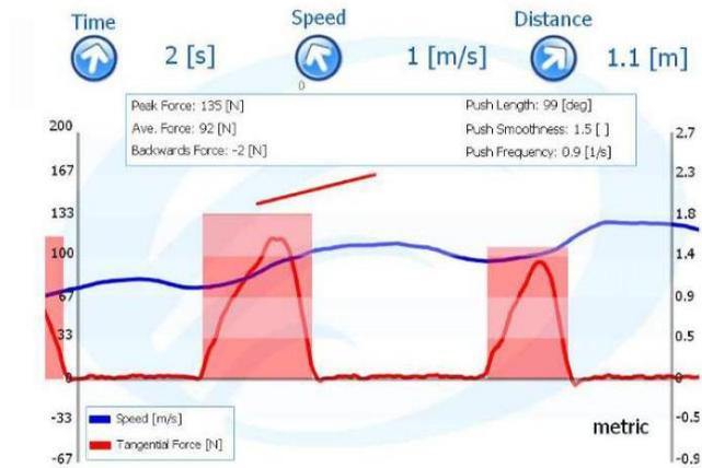
Figure 1.8 SmartWheel biofeedback interface.
