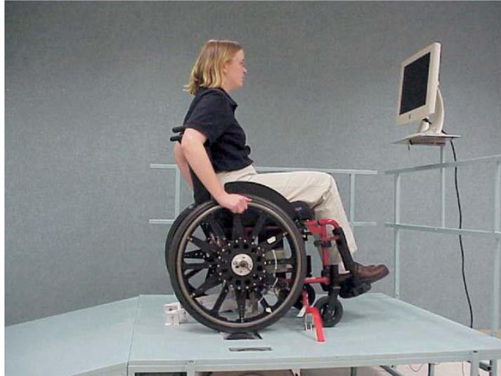
Figure 1.7 Wheelchair dynamometer with feedback on velocity, power output, and FEF.
