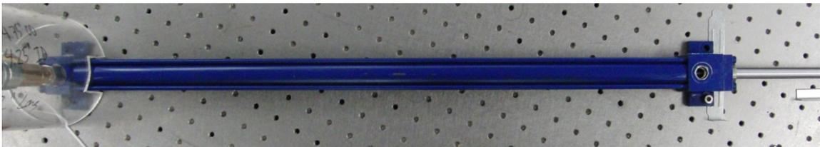
Figure 37 High Pressure Hydraulic Cylinder
