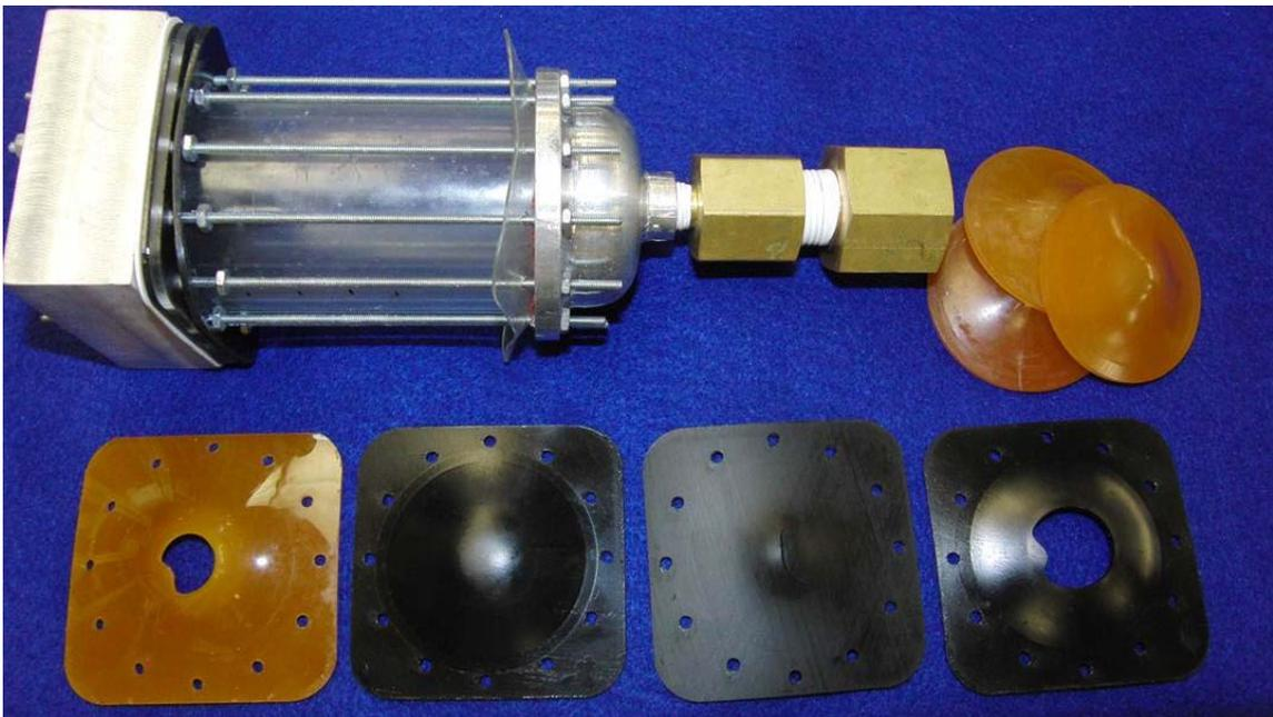
Figure 6 Post-Test Diaphragms
