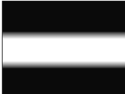
Figure 3.7: Schematic representation of an ideal tri-layer nanofiber composite membrane where the inner layer is of constant PFSA/PAI composition with a gradient composition between the inner and surface layers.
