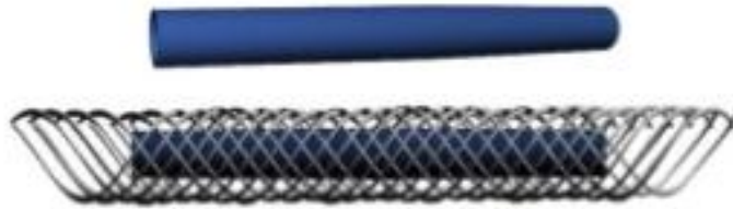
Figure 11: Skeleton of the McKibben Artificial Muscles
