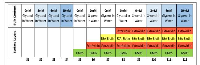
Table 2- Model 2: Each data set consisted of BSI signals obtained under 12 different conditions. This table lists the bulk fluid content of the microchannel and the surface bound molecule layers present for each of the 12 samples (S1-S12) in model 2.
