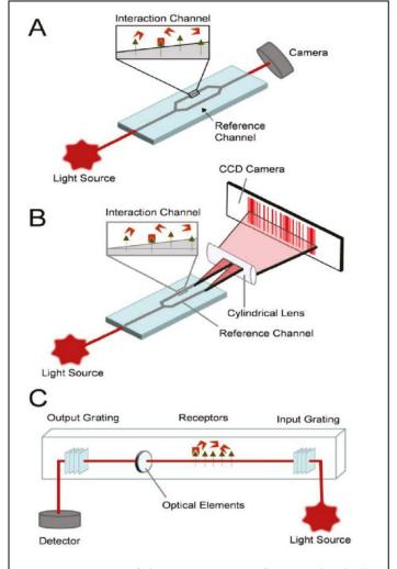
Figure 2- Schematic of A) Mach-Zehnder interferometer (MZI), B) Young interferometer (YI), C) Hartman interferometer (HI) [2]. In all three configurations, incoming light interacts in regions where analytes of interest bind and resultant phase shifts of the outgoing are measured.
