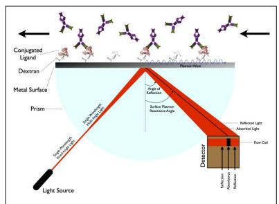
Figure 1- Schematic of Surface Plasmon Resonance (SPR) configuration [1]. A single wavelength of light is guided to a metal surface where a tethered dextran resides to bind to the analyte of interest. Light excites electrons when it makes contact with the metal, causing a plasmon wave. Analyzing reflected and absorbed light using a detector can give insight into the binding taking place on the surface.
