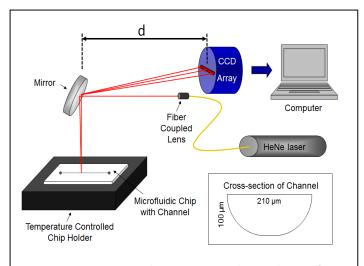
Figure 6- BSI instrument schematic. A He-Ne laser is directed from a fiber coupler to the microfluidic channel via a mirror. The backscattered light is then directed, via the same mirror, onto a CCD array camera and recorded in LabVIEW.
