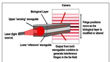
Figure 3- Illustration of a dual-polarization interferometer configuration [3]. Two planar waveguides are illuminated by the same beam of light. The polarization of the light is alternated between two modes and the resulting interference pattern is projected and measured.
