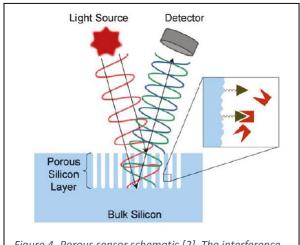
Figure 4- Porous sensor schematic [2]. The interference pattern in porous sensors results from light interacting with analytes binding to the surface inside the pores.
