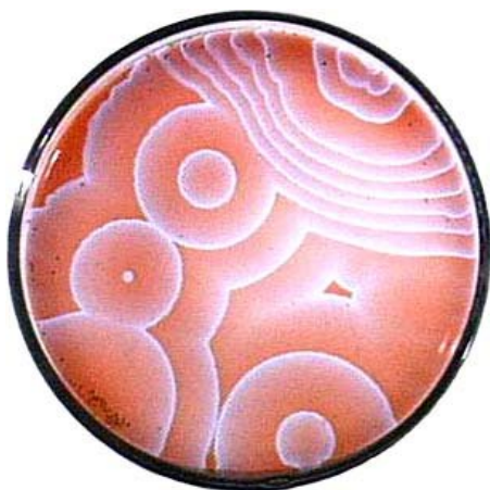
Figure 9: The wavelike chemical activity in the Belousov-Zhabotinskii reaction is shown here in a petri dish. Its chemical reaction shows a periodic color change between magenta and blue within a period of approximately one minute. It occurs with a mixture of sulphuric acid, potassium bromate (V), cerium sulphate, and propanedioic acid. The color change is caused by alternating oxidation–reductions in which cerium changes its oxidation state ( \text{Ce}^{3+} gives a magenta solution while \text{Ce}^{4+} gives a blue solution). 121 ( jchemed.chem.wisc.edu:8000/.../SP14/prog1-SP14.html ).
