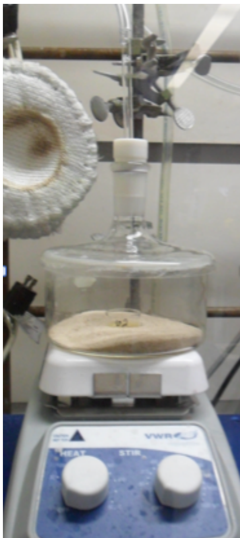
Figure 2.1. Annealing apparatus for the encapsulation of ultrasmall nanocrystals.
