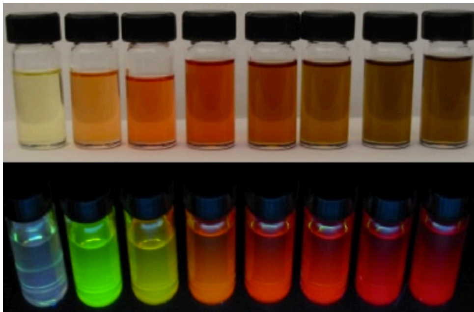
Figure 1.2. Vials of CdSe nanocrystals with increasing nanocrystal diameters from approximately 2 nm (left) up to approximately 4 nm (right). The vials are shown under room light in the top picture and are shown under UV light in the bottom picture.
