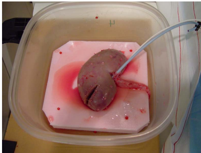
Figure 2. Porcine kidney with glass bead fiducials attached to the surface to track deformation. The kidney was perfused with saline and cut with tracked scalpel.
