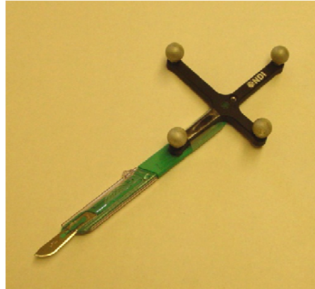
Figure 1. Scalpel with Polaris target attached to handle, used to track an incision made to the renal parenchyma.
