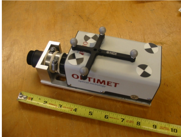
Figure 2. Conoscope with Polaris rigid body attached.
