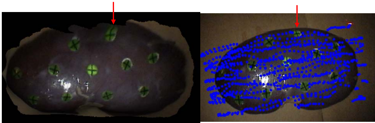
Figure 13. Examples showing the potential inaccuracy of the textured surface at the edges, due to the lack of interpolating points near the high curvature area and “bleeding out” of the texture. The red arrow shows the fiducial close to the edge that was distorted due to the lack of points.
