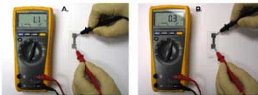
Figure 19. Resistance values for silver inks. (A) ANP silverjet nanopaste and (B) Cabot silver paste.
