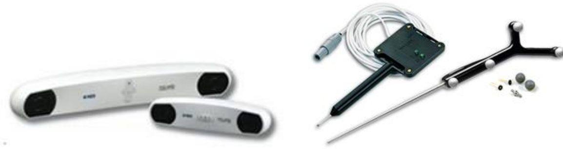
Figure 4. Northern Digital Polaris Spectra (far left) and Vicra (mid left) detectors, Polaris active emitter (mid right) and passive reflective sphere (far right) probes [ http://www.ndigital.com/medical/polarisfamily.php ]
