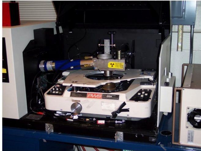
Fig. 14. 10-keV X-ray irradiator as used in the experiments.
