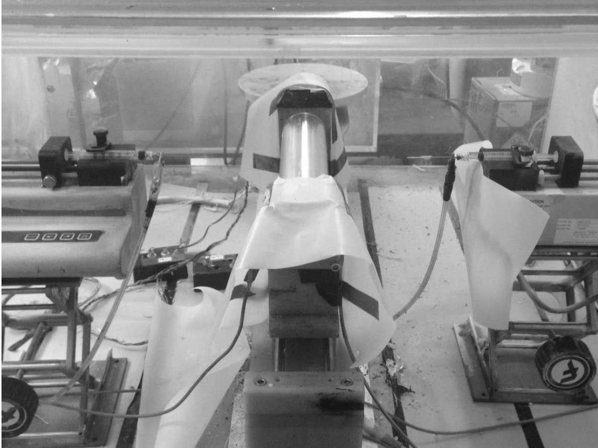
Figure 3.2. Rotating and linearly oscillating drum apparatus for dual fiber electrospinning
