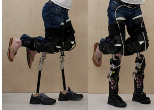
Figure 5.1: The author wearing able body adapters with the passive and powered prostheses.
