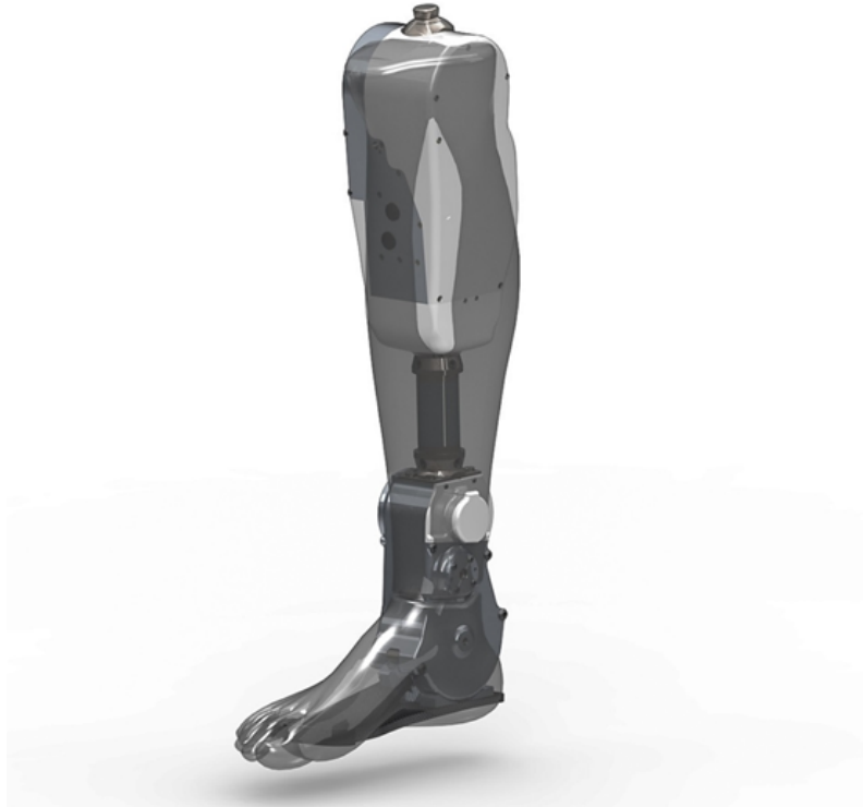
Figure 4.3: The powered prosthesis inside an anthropomorphic envelope.
