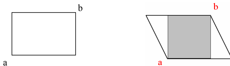
Figure 17: Original rectangle is shown on the left. On the right effect of skewing on the box defined by points a and b . The new box is presented by the gray area. White areas are lost.
