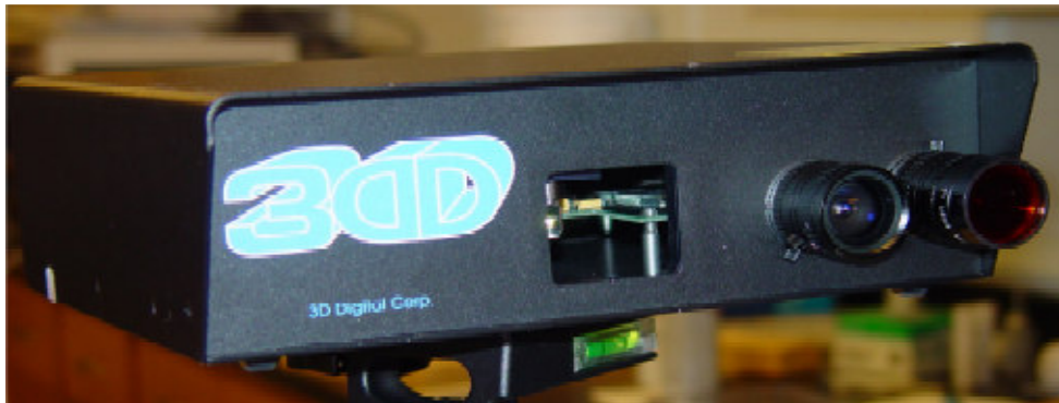
Figure 3 Laser range scanner used to obtain surfaces.
