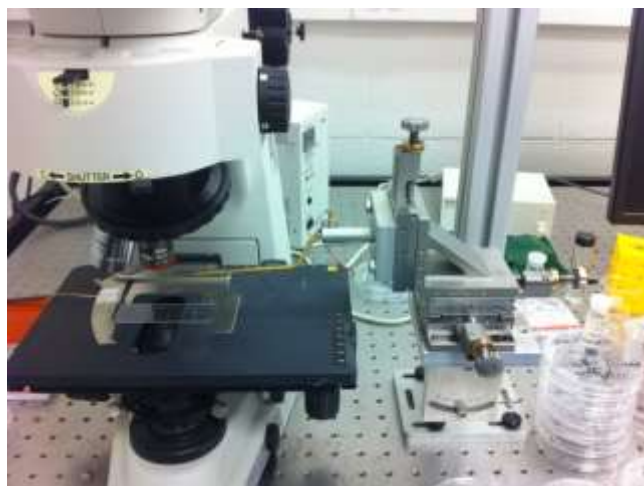
Figure 2.2 – An in-house built manipulator in conjunction with a Nikon microscope used to manipulate nanostructures.
