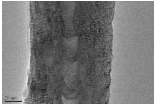
Figure 3.5- TEM micrograph of a Nanoshel sample. Amorphous carbon and defects can be clearly seen from the image, and the diameter is not well defined.
