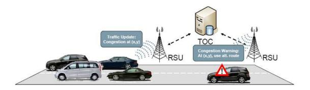
Figure ii : Traffic monitoring and Congestion Control
