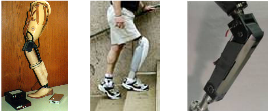
Figure 1-2. Powered knees developed by Popovic et. al. (left), Ossur (center) and Martinez-Villalpando et. al. (right).
