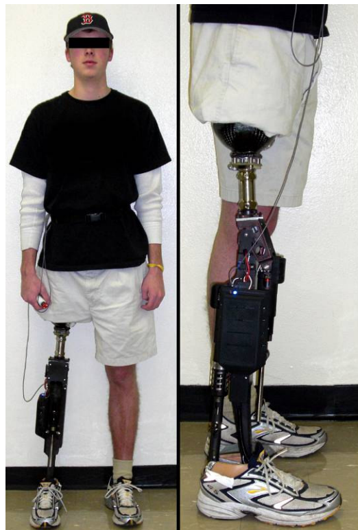
Figure 3-11. Unilateral transfemoral amputee test subject used for the powered prosthesis evaluation.
