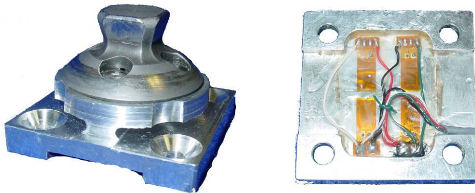
Figure 2-3. Sagittal moment load cell, top and bottom views.
