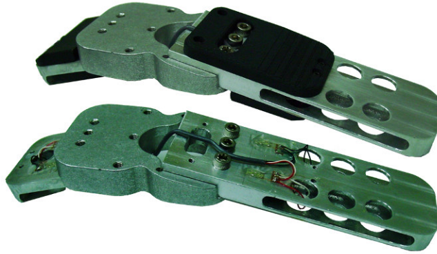
Figure 3-5. Sensorized prosthetic foot with and without strain gage covers.
