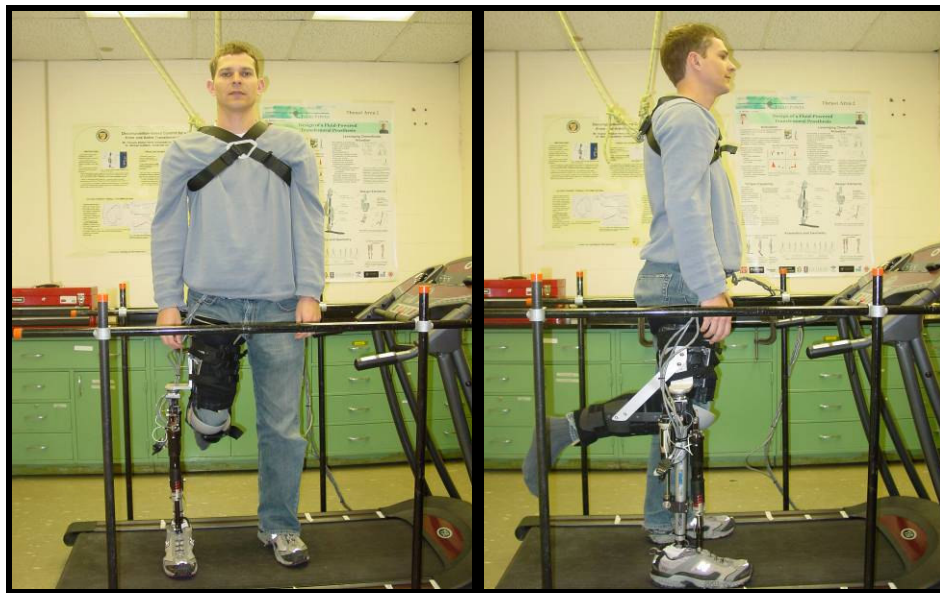
Figure 2-6. Able-bodied testing adapter used in the development of the prosthesis and controllers prior to transfemoral amputee participation.
