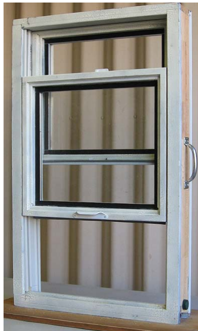
Figure 10 Portable, free-standing window used for testing, equipped with two pressure-sensitive switches in the sill to indicate if participants applied sufficient pressure, as instructed in the presentation.
