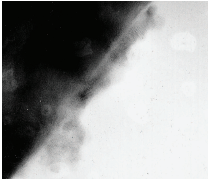
Figure 4.3: TEM of CdSe nanocrystals chemically linked to the inside wall of a TiO 2 nanotube. The large dark portion is the nanotube wall, along which individual nanocrystals can be resolved.
