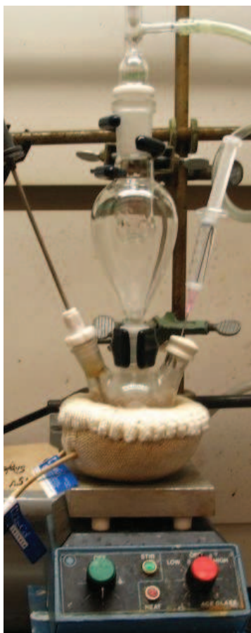
Figure 2.1: Standard nanocrystal synthesis configuration
