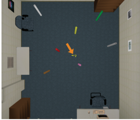
Figure V.1: This figure shows a top-down view of virtual environment that is approximately 5m x 5m. A user is instructed to examine the environment and moves his head around slightly to view the world. The head motion of the user in the virtual environment is shown in yellow (emphasized by the orange arrow). Movement in this example is 1:1, which means that movement in physical space corresponds to that same movement in virtual space.
