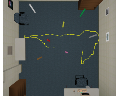
Figure V.2: This example shows the same virtual environment and user physical movement as Figure V.1. However, movement in physical space is scaled by a factor of twenty so that the small movement in physical space reflected by the yellow line in Figure V.1 becomes the yellow line in the current figure.
