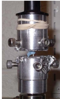
Figure 28. A murine mouse tibia loaded within the testing apparatus.
