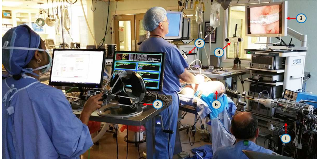
Figure 6.7: TURBot system: (1) TURBot, (2) Omega.7 master haptic interface, (3) Surgeon monitor, (4) Optical tracker base, (5) Optical marker on transvesical endoscope camera, (6) Swine
