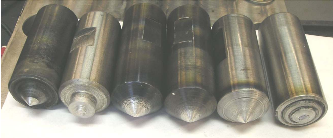
Figure 135: Tools used in the experiments (from left: 90° conical tool; cupped shoulder (5/8" diameter), threaded probe (0.20" diameter) tool; snubbed nose, cupped nose, 100° conical tool; snubbed nose, 100° conical tool; 100° conical tool; 140° spiral-cut, conical tool(Edison Welding Institute test design) ).
