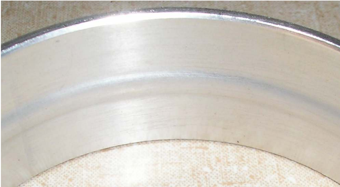
Figure 98: Bead protrusion type defect experienced in cupped shoulder ( \text{\O} 5/8'' ), threaded probe ( \text{\O} 0.20'' ) tool, bead-on-plate type welds made without a backing ring anvil. Surface quality was more difficult to maintain. ( \text{\O} = diameter).
