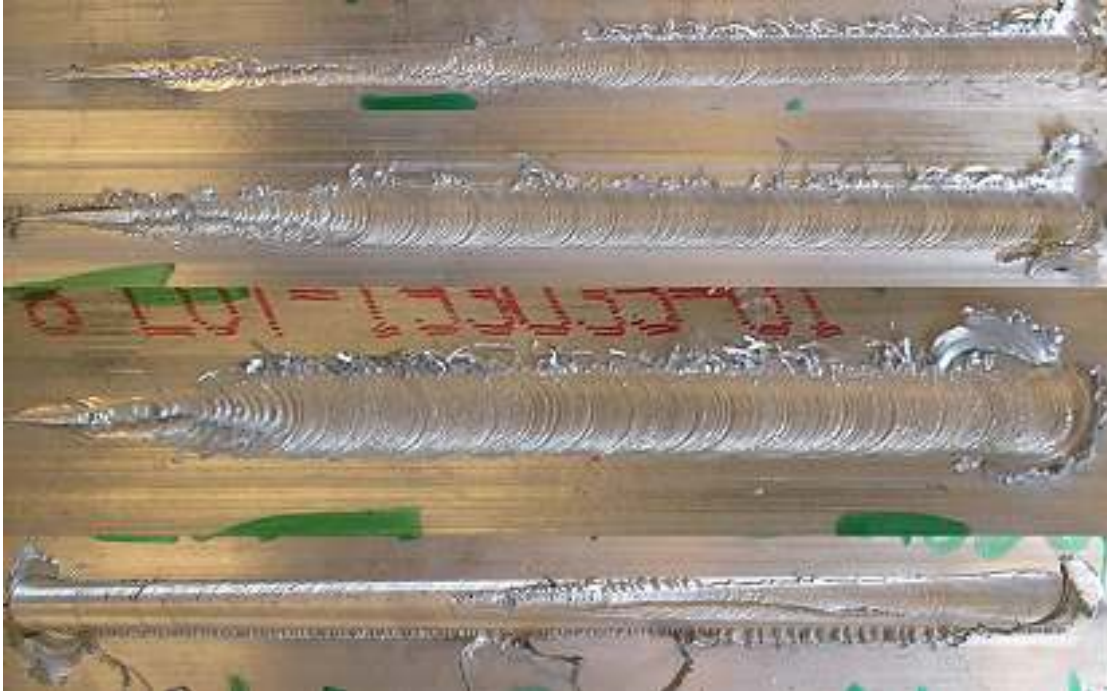
Figure 96: Attempts a probe tapered retraction from 1/8" material full penetration welds at various parameters. The probe tends to 'drag' through the material near exit.
