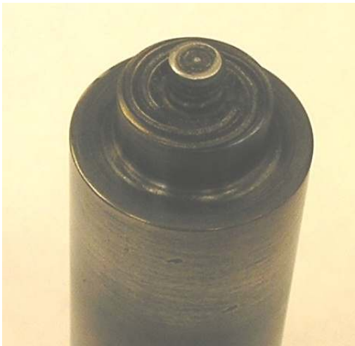
Figure 148: The 5/8" (15.9mm) diameter scrolled shoulder, 3/16" (4.8mm) probe diameter tool used in this experiment. The scrolled shoulder feature increased tolerance to variation in contact condition and improved weld appearance.
