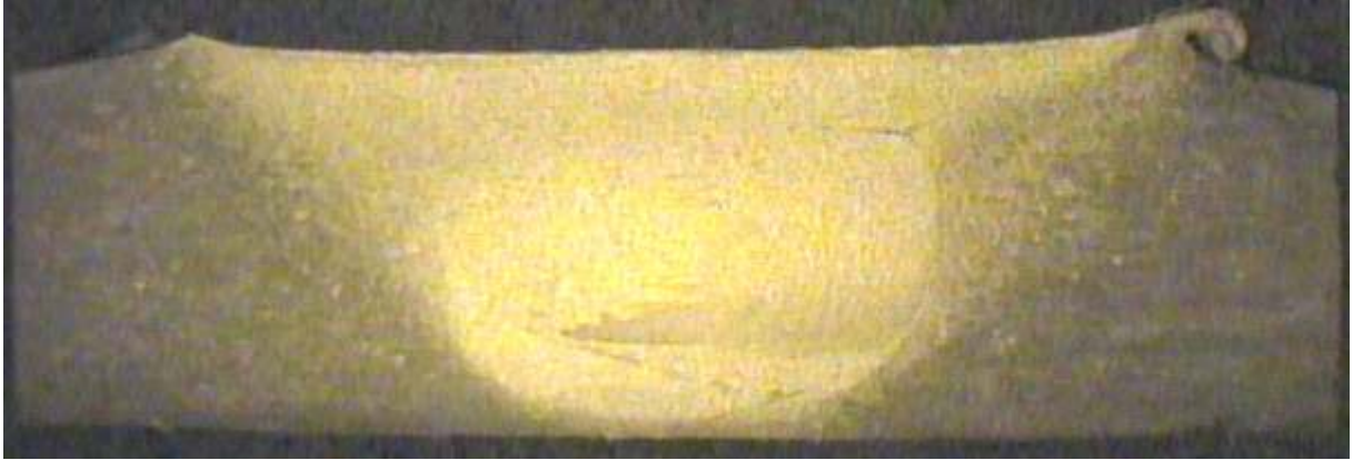
Figure 131: (threaded tool) Lateral macrosection corresponding (1000rpm, 7.8ipm) to the CFD simulated weld showing the TMAZ(bright), parent metal(dark), and transitional HAZ (intermediate). The HAZ region can be compared to isotherms in Figure 129 and the TMAZ or stirred zone can be compared to the velocity magnitude contour in Figure 130.
