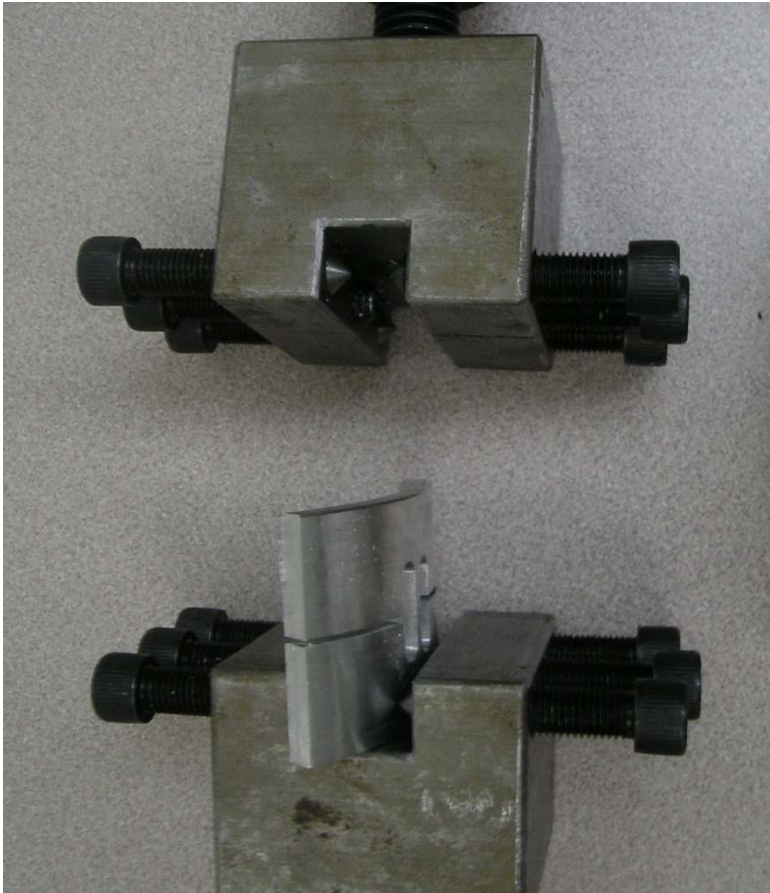
Figure 143: The curvature of the pipe tensile coupons required the use of specialized clamps. The tensile jaws pictured above were designed to grip tensile coupons cut from welds of butted pipe and butted hemisphere sections. Each jaw uses six bolts to grip each coupon. Bolt tips are spiked, snubbed, or flat depending on the geometry gripped and the location contacted on the coupon.
