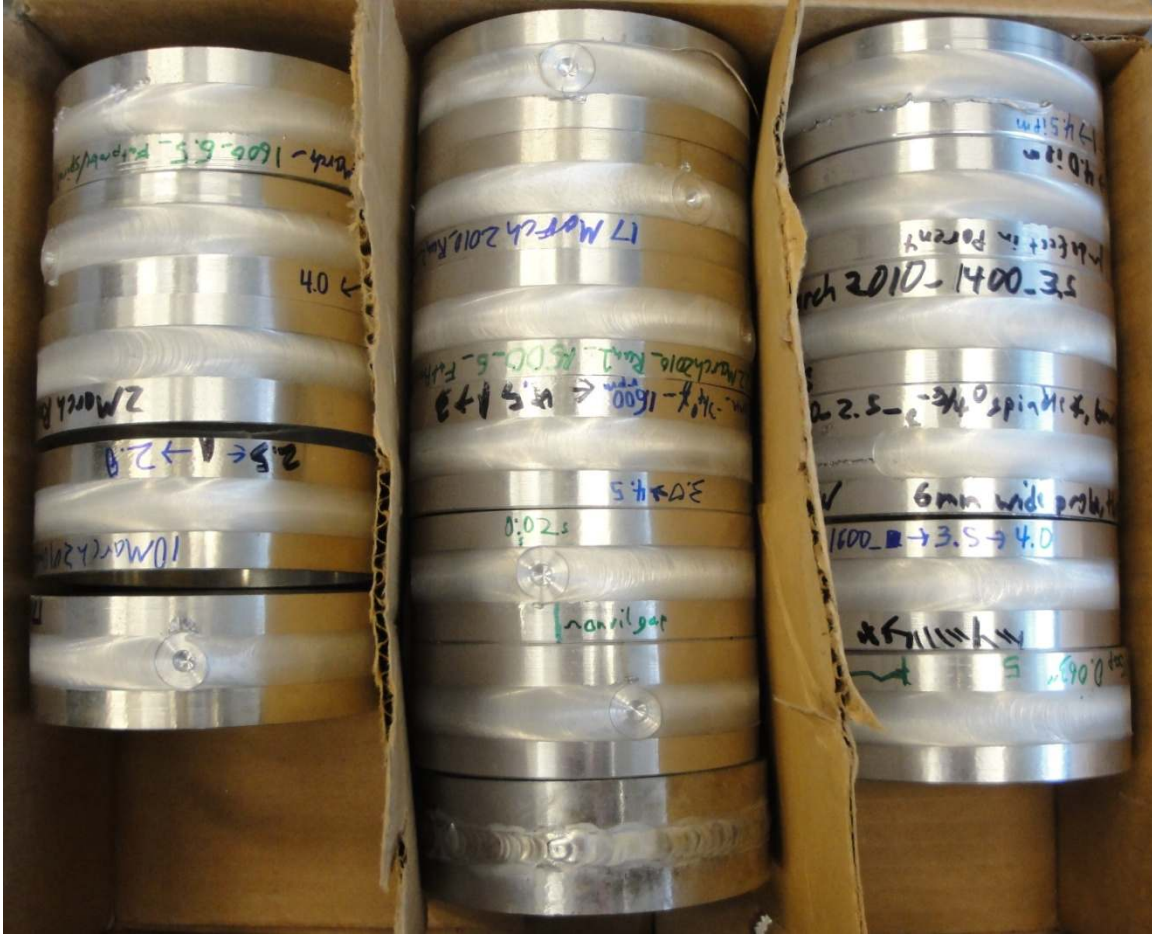
Figure 179: The superficial appearance of some of the pipes welded in the experiment and some additional pipe welding runs not presented in the experiment. The center and bottom sample is a tungsten inert gas, TIG, weld made for comparison with filler type 5356.
