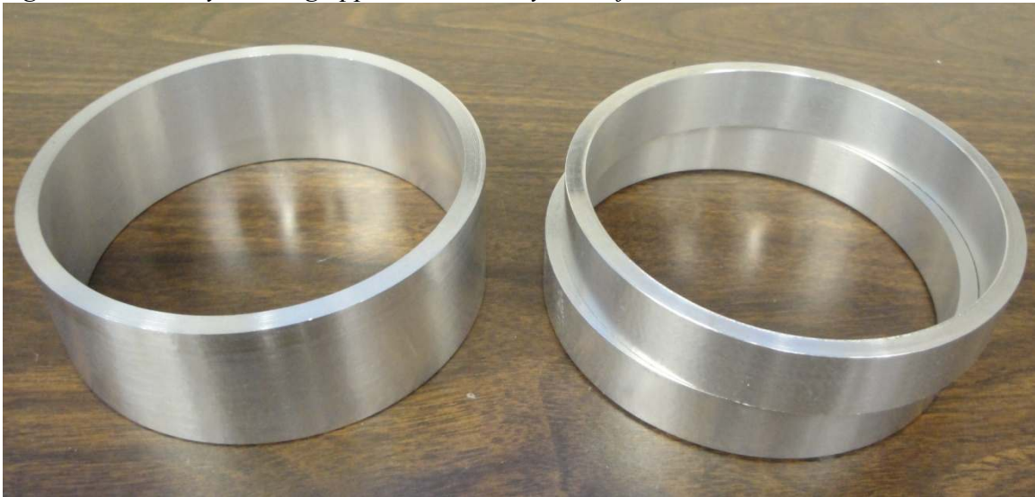
Figure 184: Left is a pipe sample used for tensile coupons of the parent material and geometry. Right are pipe sections joined in the experiment.
