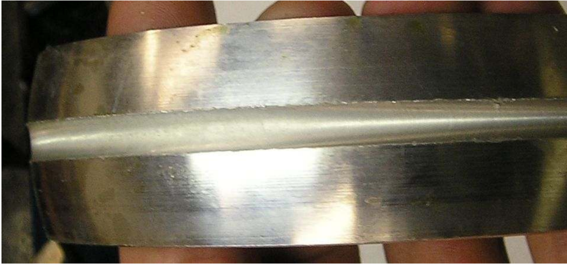
Figure 101: Surface appearance for a butt configuration weld made with a 100° conical tool (Ø 0.025” snub-nose and Ø 0.015” cupped nose recess). No backing ring anvil was used.
