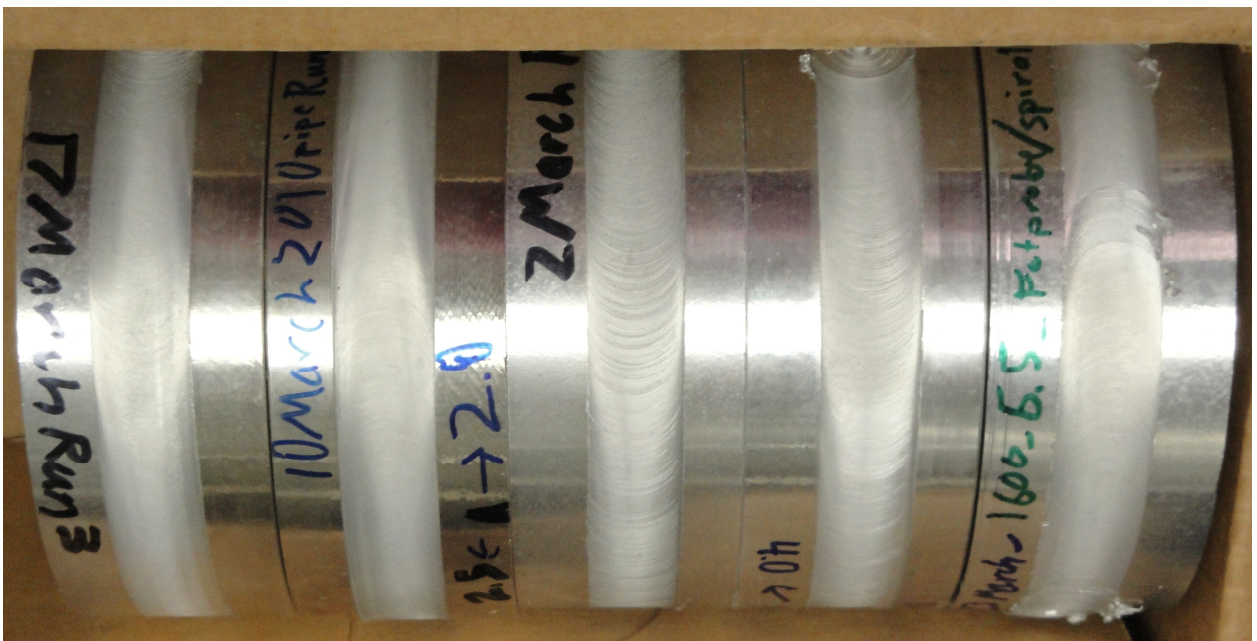
Figure 150: The superficial appearance of several pipes welded in the experiment.
