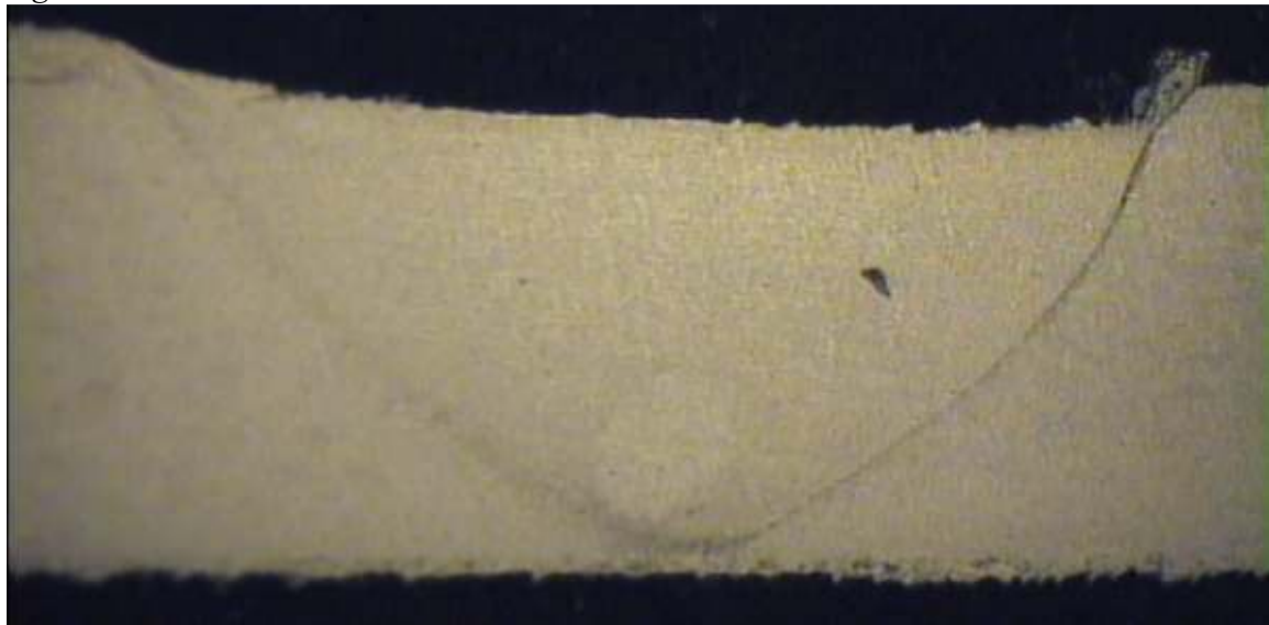
Figure 76: Macrosection of the strongest conical weld (90°, 1600rpm, 4ipm, Run#1). A minimal penetration ligament is crucial to weld strength. Failure in the tensile coupon occurred along the retreating (right) side weld nugget boundary.
