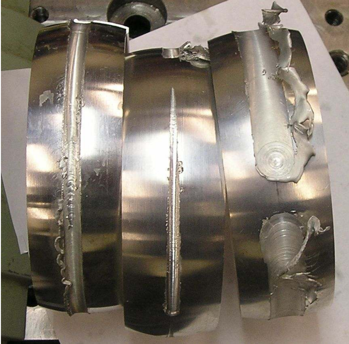
Figure 136: (from left: Tapered retraction over welded material ( 100^\circ snub-cup); bead on plate tapered retraction ( 100^\circ snub-cup); 0.09" depth weld made with a 140^\circ spiral-cut, conical tool).
