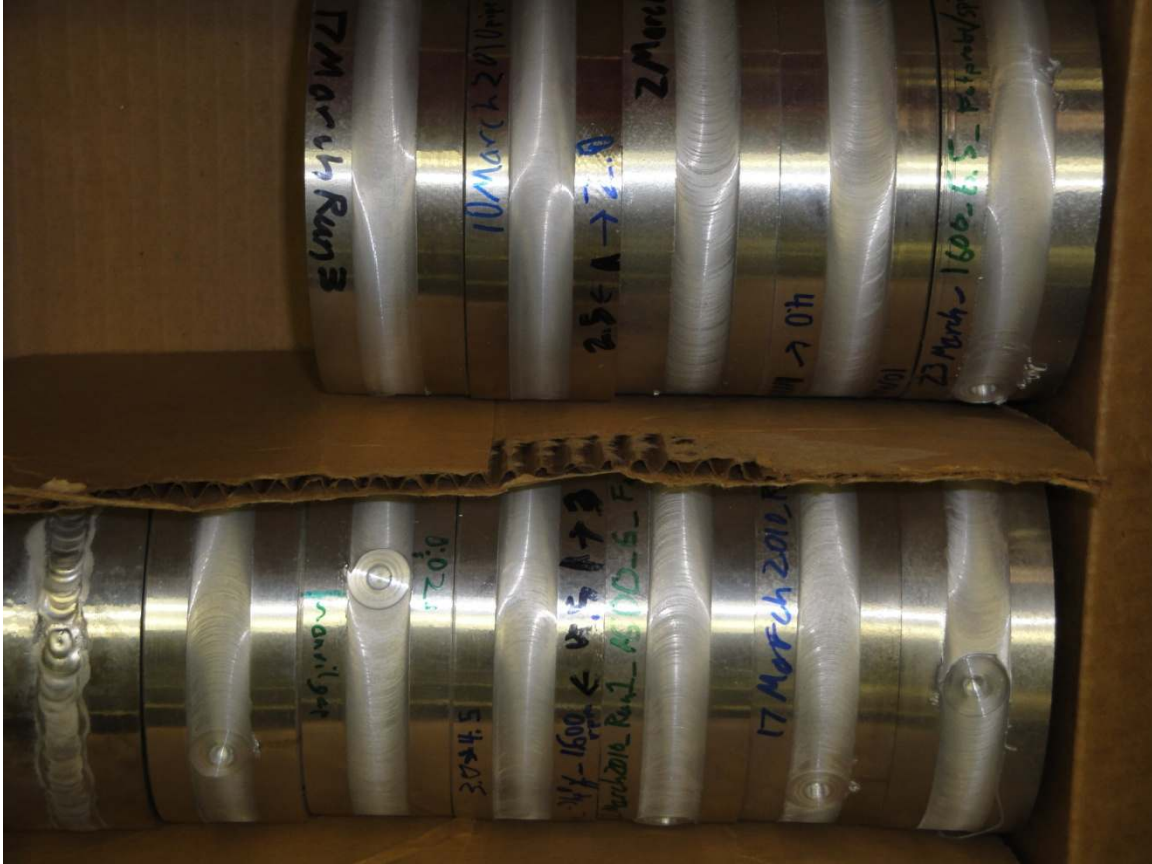
Figure 181: The superficial appearance of some of the pipes welded in the experiment and some additional pipe welding runs not presented in the experiment. Left and bottom is a TIG weld sample.
