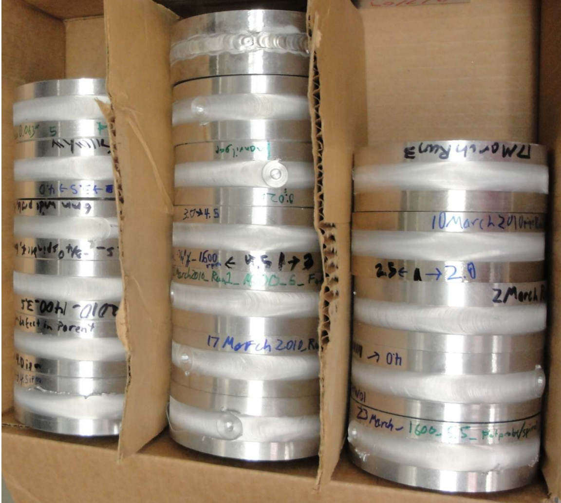
Figure 180: The superficial appearance of some of the pipes welded in the experiment and some additional pipe welding runs not presented in the experiment. The top and center sample is a TIG weld.
