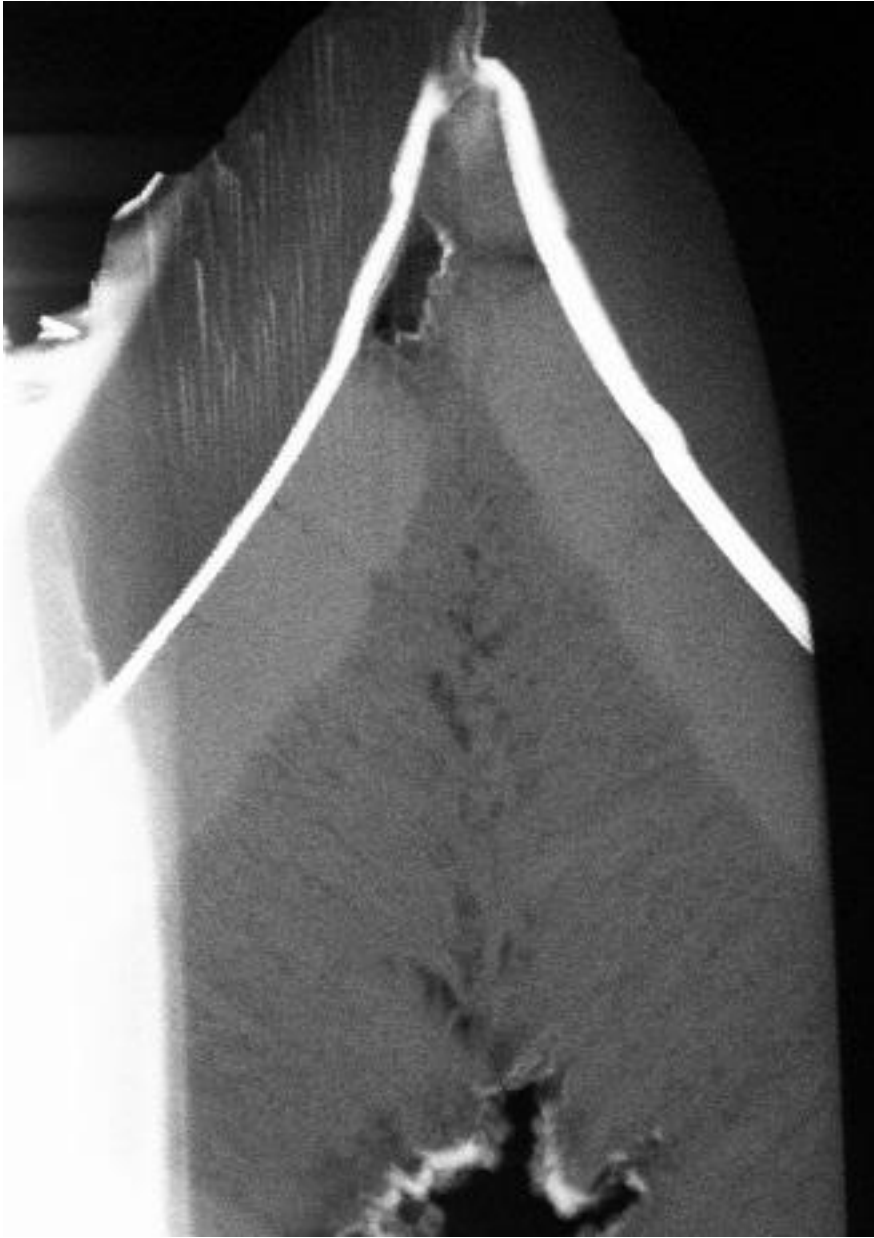
Figure 4-19: HAADF TEM of a tip with high contrast observed between the microdiamond and nanodiamond layers which was observed by TEM to correspond to increased graphitic content in the microdiamond layer.
