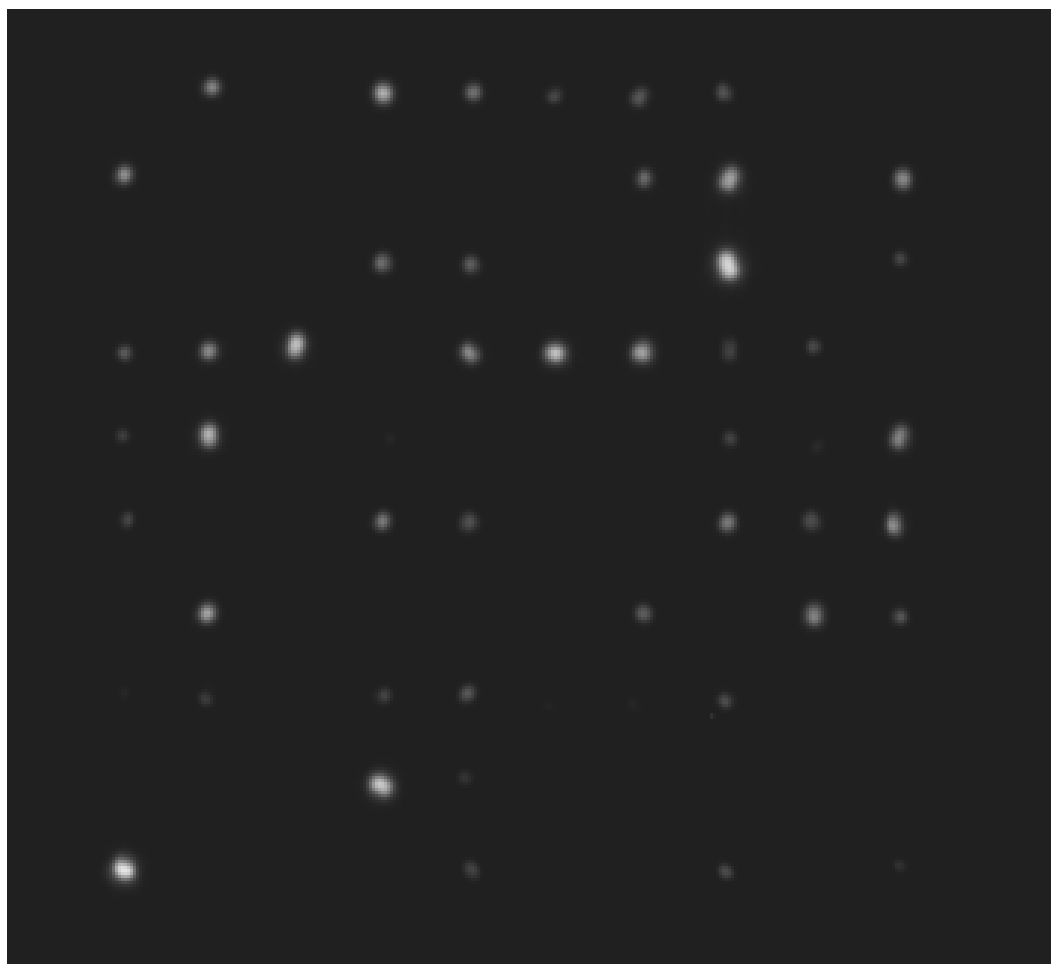
Figure 4-8: Visible light field emission image on phosphor.
