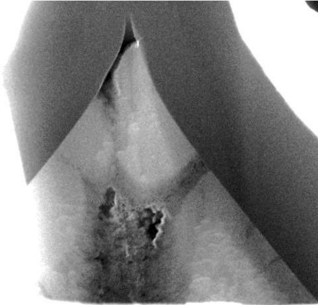
Figure 4-17: TEM image from 100 tip correlational array, Tip 2. The apex appears to be missing, and we observe very large nanodiamond nucleation colonies.
