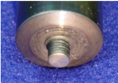
Figure 6.4: FSW tool used for torque control.
