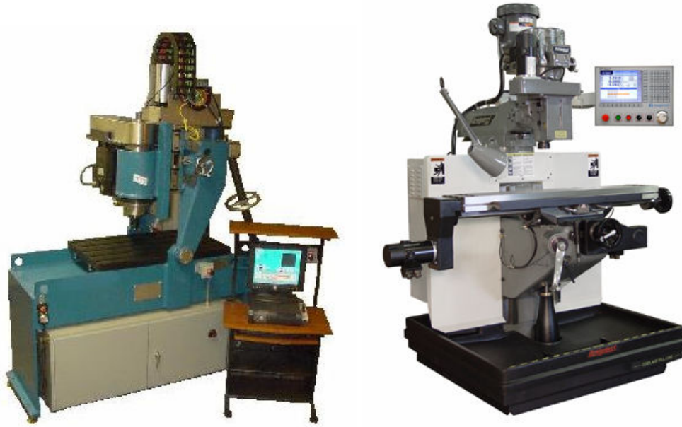
Figure 1.16: A Transformation Technologies Inc. RM-1 FSW machine (Transformation Technologies, Inc 2009) and a Bridgeport EZ Vision CNC mill (Hardinge 2009).
