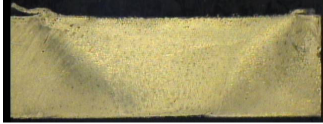
Figure 4.12: Cross section of a weld seam, example 2.
