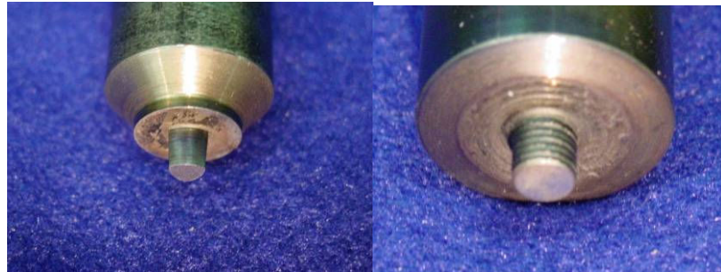
Figure 5.4: Trivex and threaded FSW tools.
