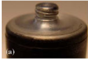
Figure 1.9: Basic FSW tool configuration (Atharifar et al. 2007).
