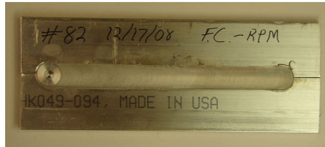
Figure 5.14: Weld sample of force control via rotation speed.
