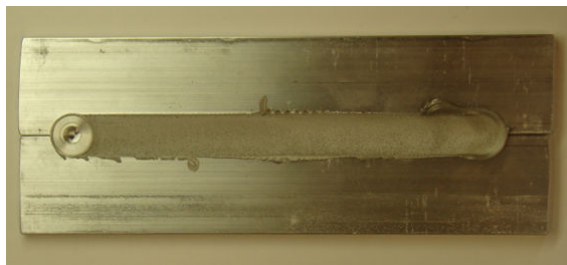
Figure 5.13: Weld sample of force control via traverse speed.
