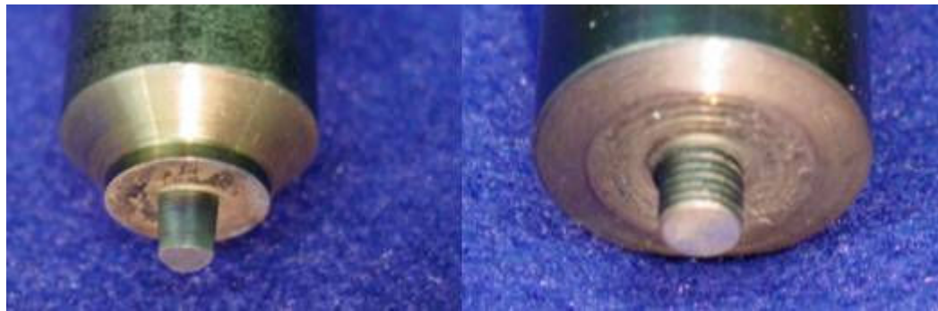
Figure 3.3: Trivex and threaded FSW tool.
