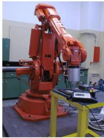
Figure 1.18: Robotic FSW setup by Smith (2000).
