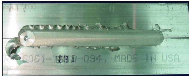
Figure 5.6: Welding without force control.
