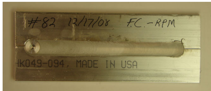
Figure 4.6: Welded sample using force control via rotation speed.
