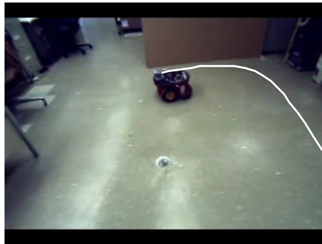
Fig. 5.10: Pioneer P3DX trajectory on slippery surface after the application of dynamic planner
