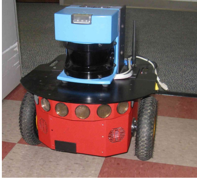
Fig.5.11: Pioneer P3DX with mounted laser measurement sensor
