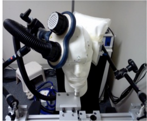
Figure 3. Demonstration of TMS Coil Positioned Over a Mannequin Head
