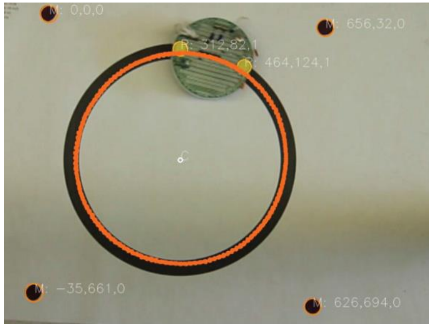
Figure 58. Image after video processing, showing the track the robot followed in orange. This is an example of successful tracking.
