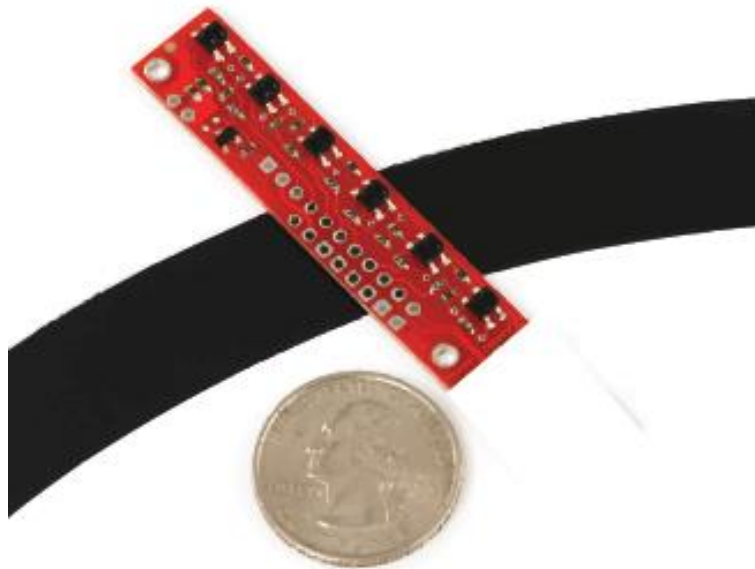
Figure 35. Image of line sensor over a track [66]. In operation the line sensor faces the track. The outputs from each of the six sensors are combined in a weighted function to create a single input signal to the robot control system, as shown in Figure 36.
