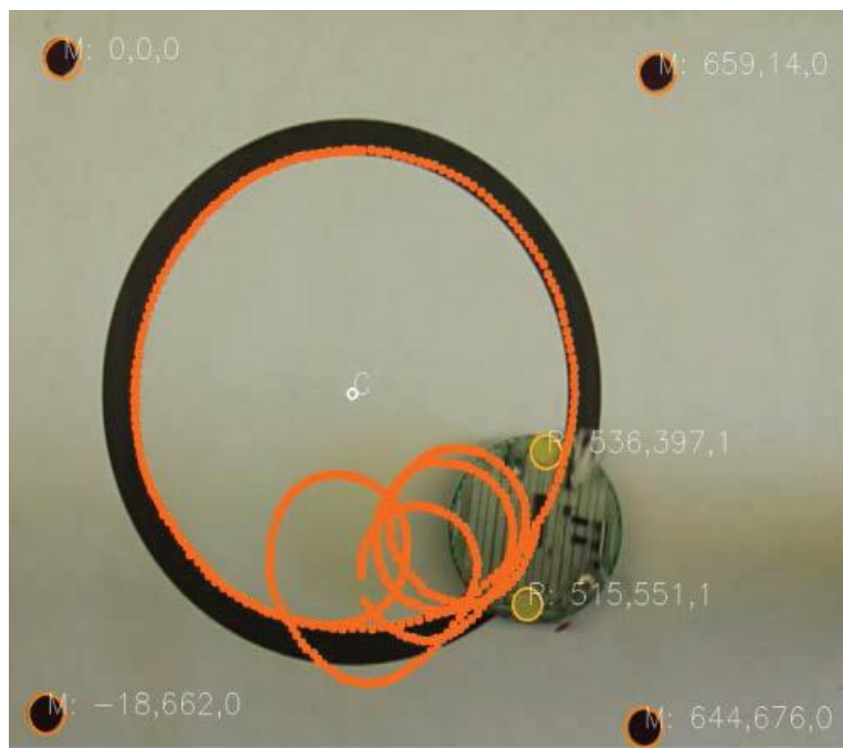
Figure 59. Image after video processing. This is an example of failed tracking, with the robot spiraling in circles near the bottom of the image.
