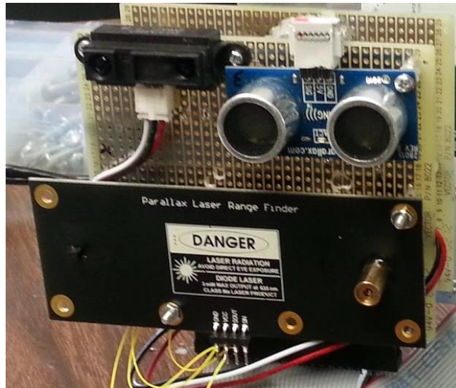
Figure 5. Photograph of the three types of rangefinders tested on the mount used for measuring the transfer functions. From top left clockwise: IR rangefinder, sonar, laser rangefinder.
