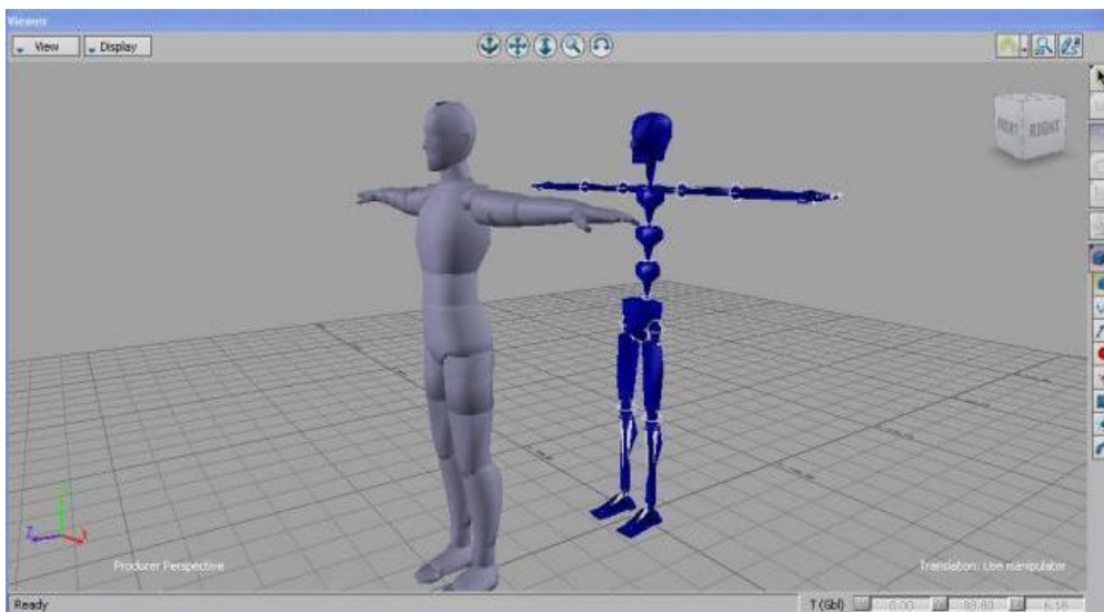
Figure 3. Data received from Vicon (represented by the left avatar) and the avatar generated by the inverse kinematics mapping (the right skeleton). Note: The two character are usually coincident in the real experimental procedure.
