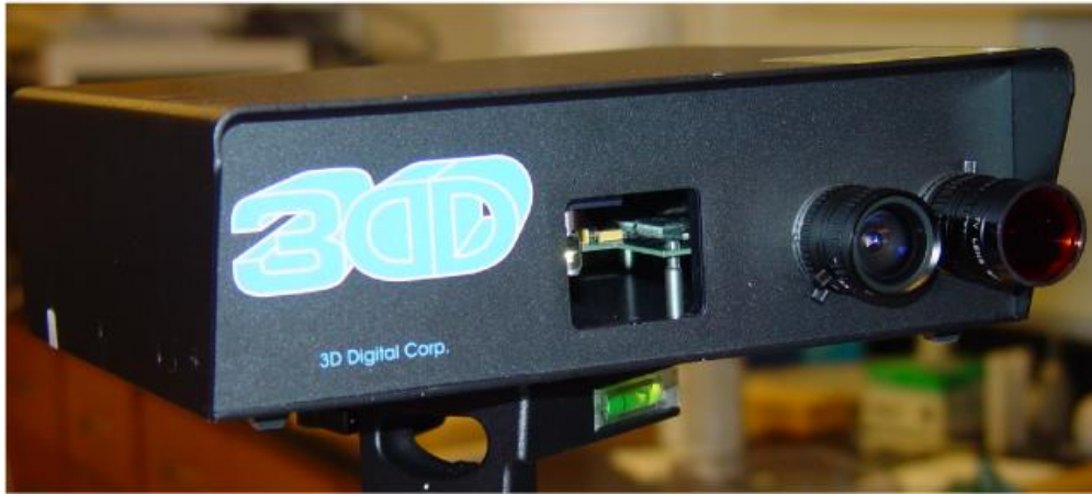
14(a) Close up of the scanner showing the laser emit window in the middle and the CCD and laser receive cameras on the right.
