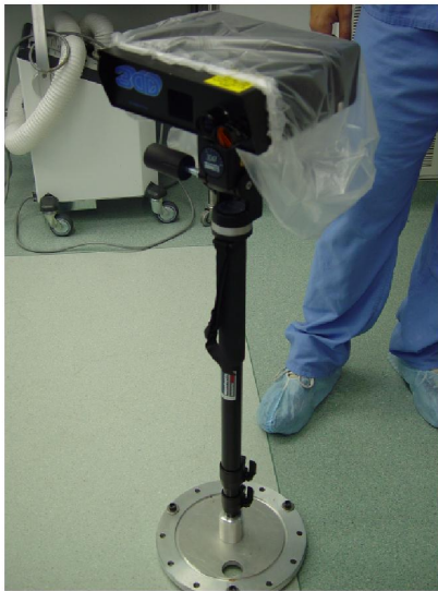
14(b) LRS in the operating room covered with sterile isolation bag and mounted on custom built vibration damping monopod.
