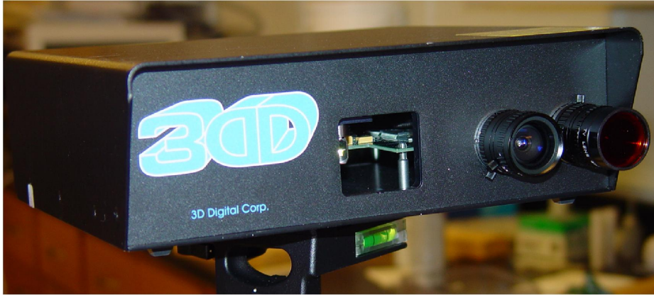
Figure 6: Laser scanner used to acquire textured point clouds.
