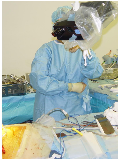
14(c) LRS in the OR, covered in sterile bag, and mounted to overhead swing arm.
