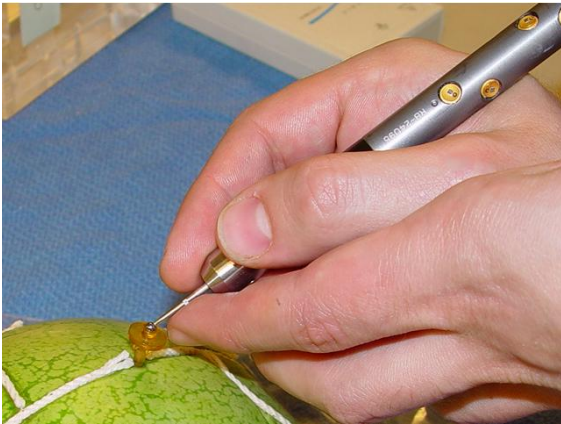
16(c) Acustar® divot caps for localization using Optotrak®.
