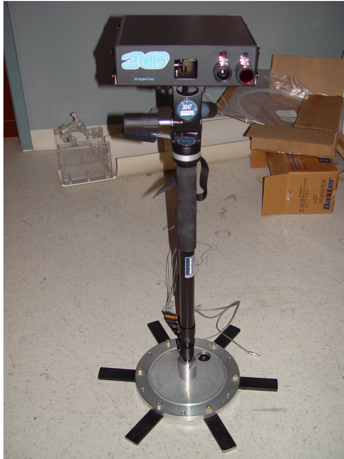
Figure 25: RealScanUSB 200 LRS device used to acquire textured point clouds of the intra-operative brain surface mounted on a vibration damped monopod.
