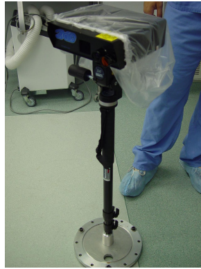
Figure 50: Laser range scanner mounted on vibration damping monopod in OR.
