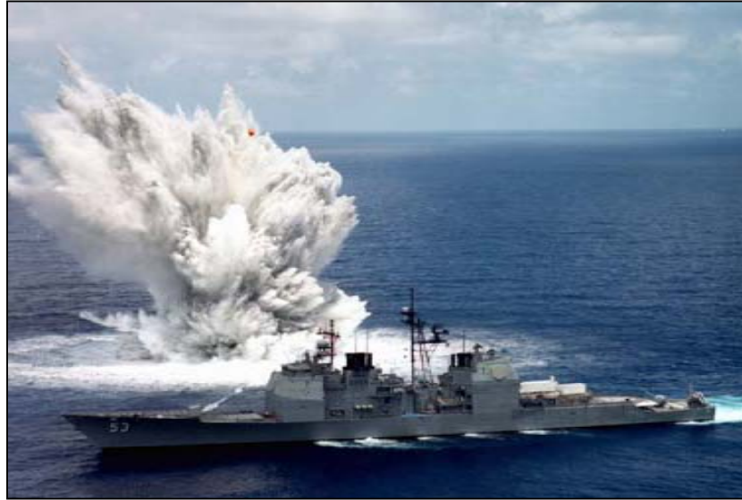
Fig. 1.2 Unique naval environment (blast loading due to underwater explosion) poses challenges to design of composite ships.
