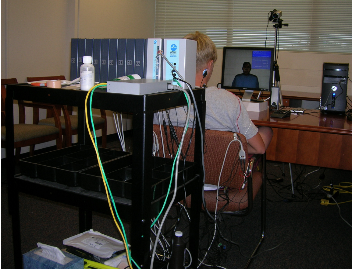
Figure 5.2 Photo of a participant sitting in front of the VR task computer; printed with permission. The Biopac MP150 equipment and amplifier modules for each physiological sensor sit on top of a black cart in the foreground.
