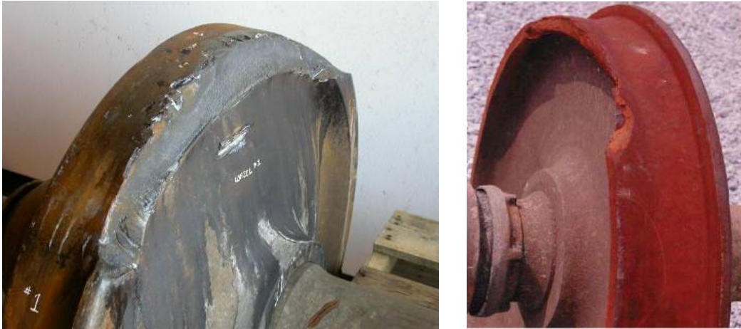
(a) (b) Figure 2. Typical vertical split rim failures [10]
