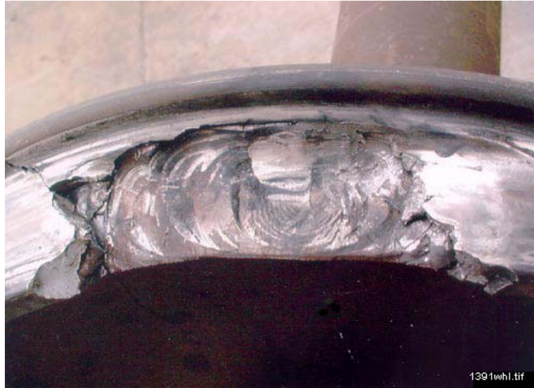
Figure 1. Typical shattered rim failure [7].
