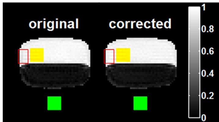
Figure 2.19. SNR improvements in fat-water phantom after k-space misalignment correction.
