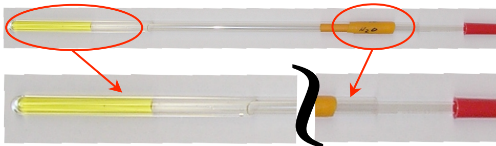
Figure 6-1: Dual NMR sample tube arrangement. Top: the 3 mm (or 4 mm) NMR tube contains the sample, a tape provides stability for the upper tube part. Bottom: the smaller tube is inserted into a 5 mm NMR tube, containing deuterated solvent.
