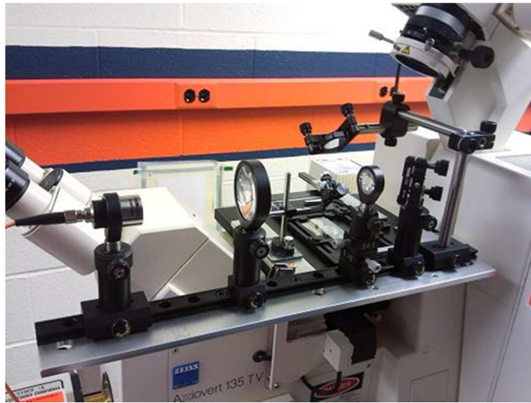
Figure 2.8: The bright-field illumination system mounted on the microscope. The fiber output coupling lens is on the left and can be replaced with the diode laser. Two mirrors on the right direct the beam on to the sample. A hydrophone used to measure pressure waves in liquid can be seen in the center, behind the two lenses forming the beam expander.
