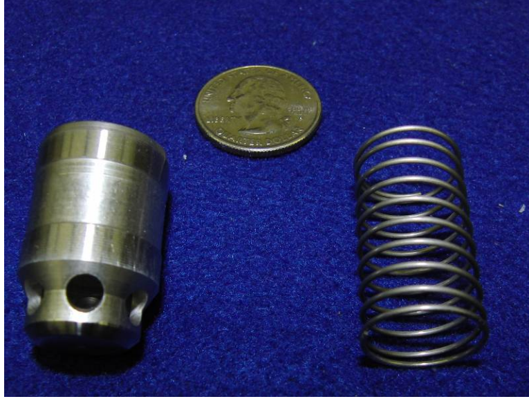
Fig. 3-7. Pump check valve piston and spring
