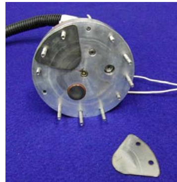
Fig. 5-10. (a) Injectors mounted to combustion head. (b) Injector check valve flaps
