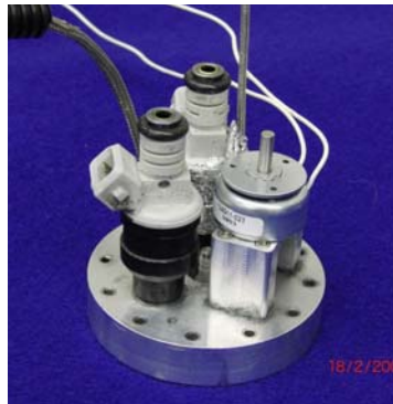
Fig. 5-10. (a) Injectors mounted to combustion head. (b) Injector check valve flaps
