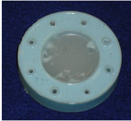
Figure 2-3. Silicone diaphragms for liquid piston
