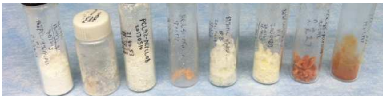
Supplementary Figure 6: Appearance of x%PCL-y%ACPCL, from left to right, in order of increasing ACPCL content.
