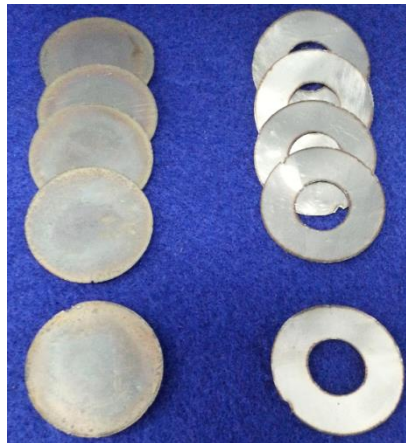
Figure 1.16 - Collapsible, in-piston heat exchangers used in hot side (left) and cold side (right)
