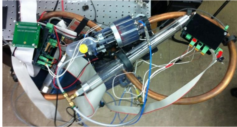
Figure 5.1 - Picture of Free Piston Compressor Engine with figure-8 high inertance liquid piston and onboard electronics and control.
