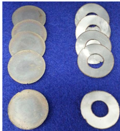
Figure 6.6 - Collapsible, in-piston heat exchangers used in hot side (Left) and cold side (right)
