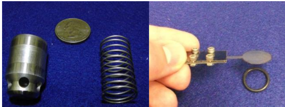
Figure 5.9 - (a) Previous Compressor Head Check Valve (b) Current Compressor Head Check Valve
