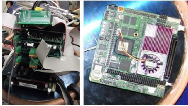
Figure 5.11 - a) On Board Electronics b) Athena Single Board Microprocessor
