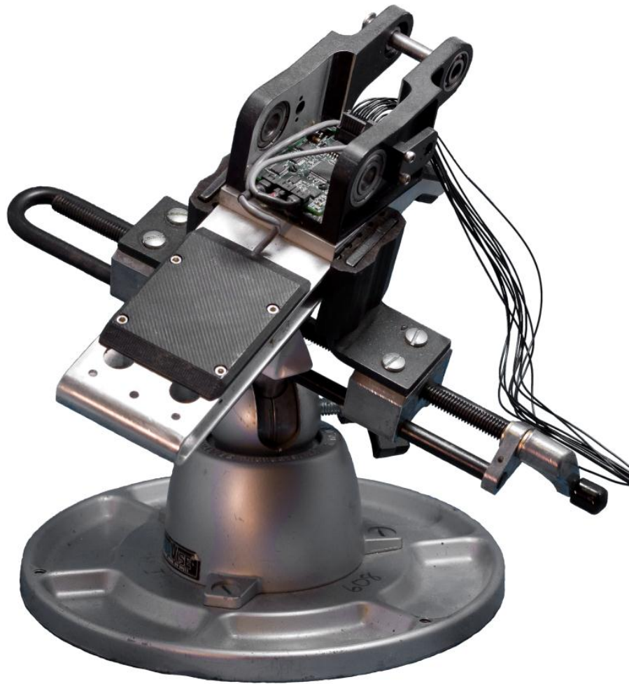
Figure III-4: Prosthetic foot clamped in vice for IMU calibration
